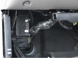
Once the PCM is removed, pull the PCM from the case making sure not to lose the metal ground tab next to the lower bolt hole of the case. We will not be using this tab but you may want to keep it if you ever decide to return the PCM back to stock configuration.
